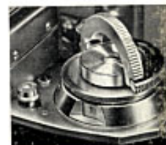
Counter of BX. Pressing a button after closing back sets counter in position.
