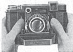
Closing the camera: Press the upper arms of the struts (13), at the same time raising the baseboard.
